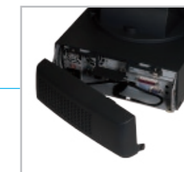
Rear cable cover for safety and neat outlook
