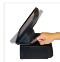
Gear button to adjust LCD swivel angle from 0° to 16° horizontally
