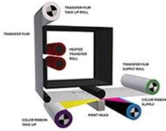
Traditional direct-to-card printers use a printhead that prints through a ribbon directly onto the card. Retransfer printers print onto a flexible, transparent film that is then thermally bonded to the card creating a more durable, scratch-resistant product. This retransfer technology produces images with optimal quality that are more vibrant and saturated, even on uneven card surfaces such as key tag or smart cards.
